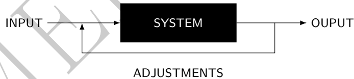
Fig. 2. High Level Diagram of the Black Box Testing Methodology [4]
